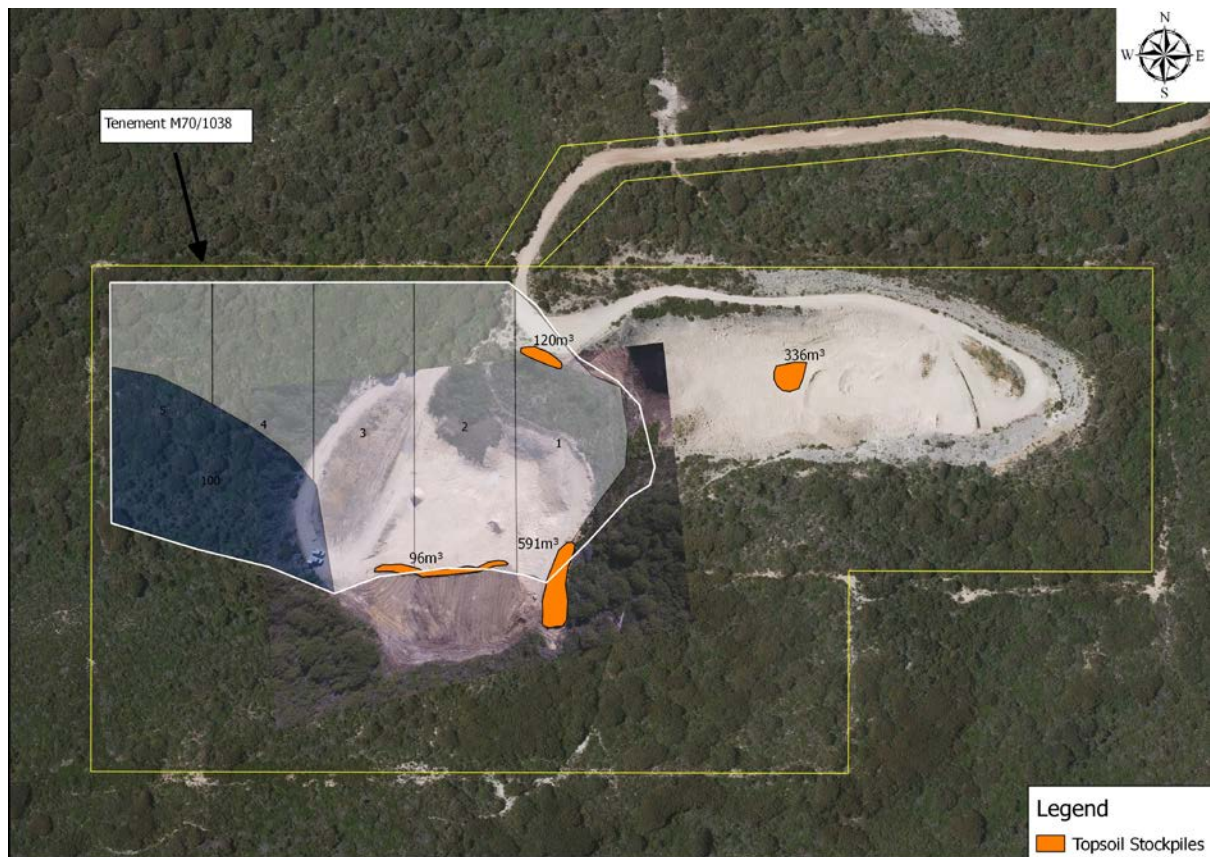
Figure 4: Location of Topsoil Stockpiles and Volumes
