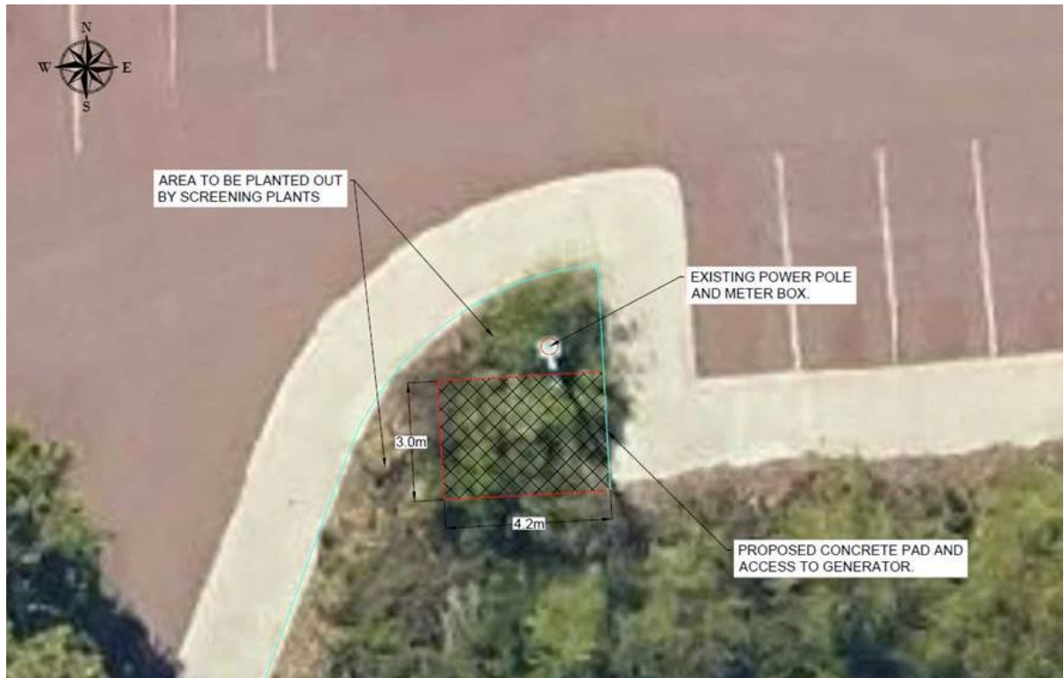
ABOVE: close up of generator location and area to be revegetated for screening.
