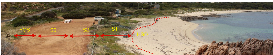
Figure 1: Concept for the assessment of coastal processes allowances under SPP2.6 as applied to Gracetown Beach for Augusta Margaret River CHRMAP.
