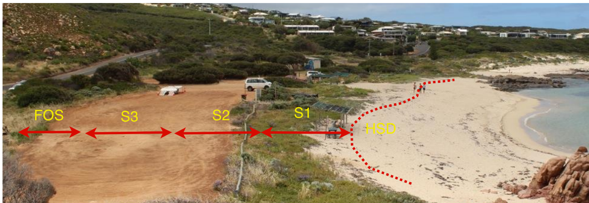
Figure 2.1 Representing Allowance for Erosion on Sandy Coast (incl HSD) S1 + S2 + S3 + FOS
